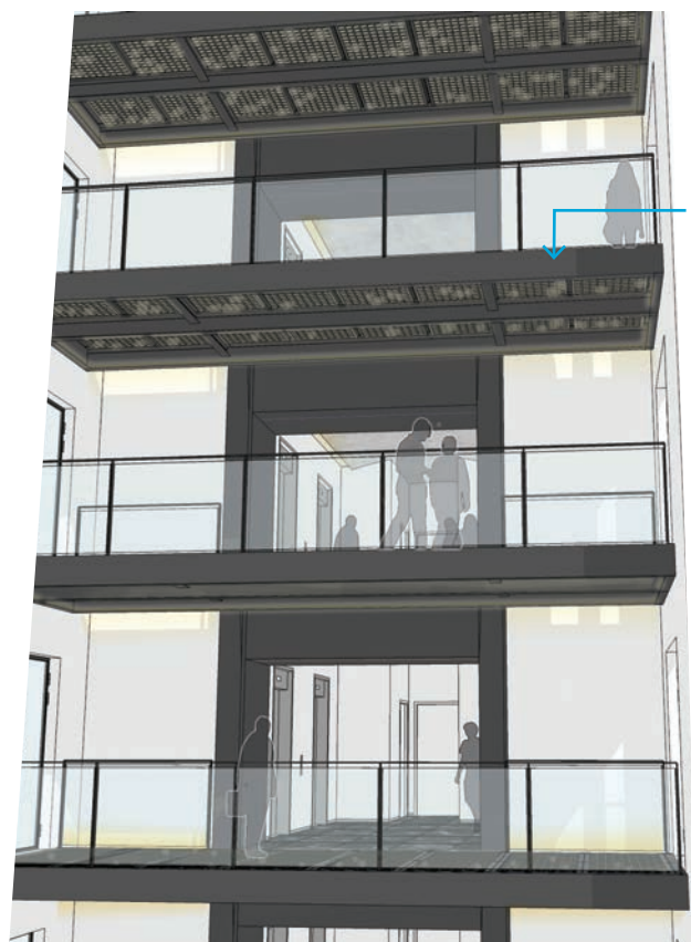
New metal bridges linking office space across Atrium (7 bridges in North Atrium, 7 bridges in South Atrium)
